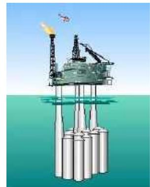
The 24 cells and 4 shafts referred to above are shown to the left while at the sea surface. The cells are 12m in
