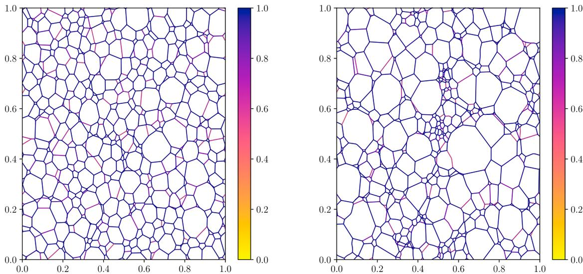
Fig. 14. Grain boundary network for  $\kappa = 1$  (left) and  $\kappa = 10,000$  (right) for Read-Shockley with  $\delta = 0.5$ . The colorbar show the corresponding value of the grain boundary energy for each boundary.
