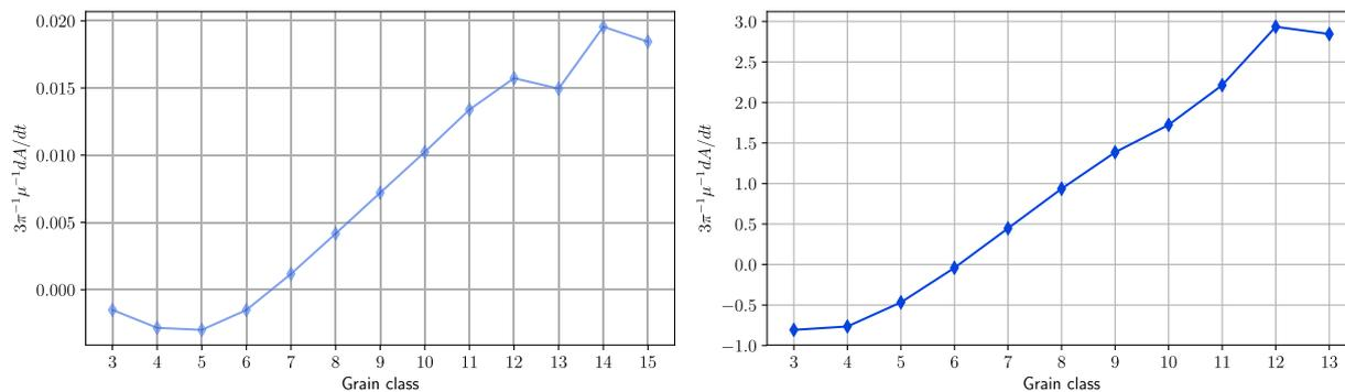
Fig. 16. Rate of change of area per grain class. (Left) Mean of  $dA/dt$  for  $\kappa = 1$ . (Right) Mean  $dA/dt$  for  $\kappa = 1000$ . This was computed by removing less than 10% of extreme values per class. This uses the Read-Shockley grain boundary energy.
