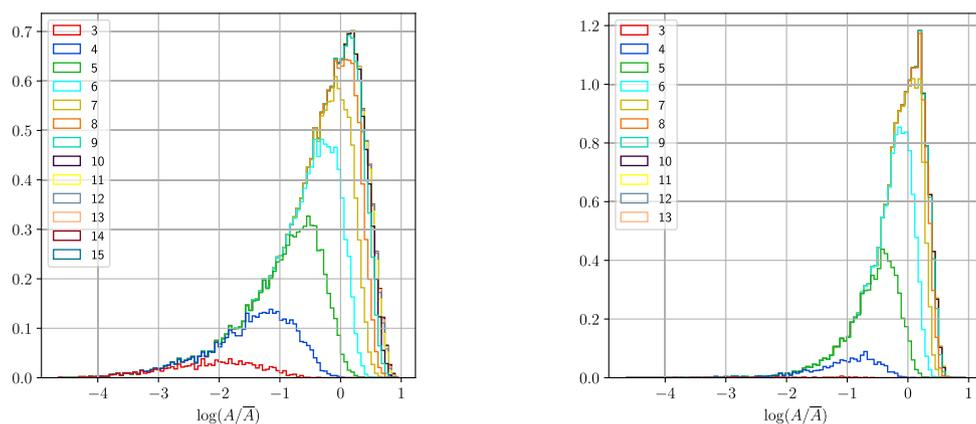
**Fig. 11.** Relative grain area distributions showing each class independently. The figure on the left corresponds to the numerical experiment performed with  $\kappa = 1$  and the figure on the right corresponds to  $\kappa = 10,000$ . In both cases we used  $\epsilon = 0.2$  for the grain boundary energy. For the cases with  $\epsilon = 0$  and  $\epsilon = 0.02$  the figures look alike so they were not included.
