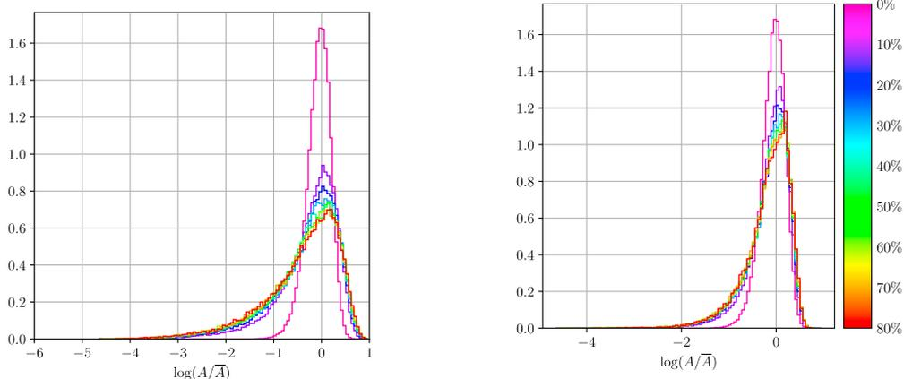
Fig. 12. Evolution over time of relative grain area distribution. The figure on the left corresponds to the numerical experiment performed with  $\kappa = 1$  and the figure on the right corresponds to  $\kappa = 10,000$ . In both cases we used  $\epsilon = 0.2$  for the grain boundary energy. For the cases with  $\epsilon = 0$  and  $\epsilon = 0.02$  the figures look alike so they were not included. The colorbar represents the percentage of grains removed.
