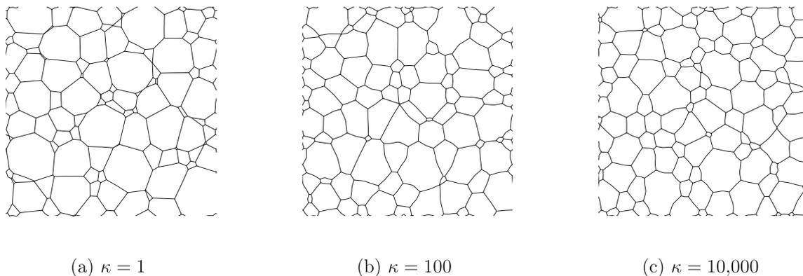
Fig. 5. Grain structures under different parameters from 1000 initial grains.
