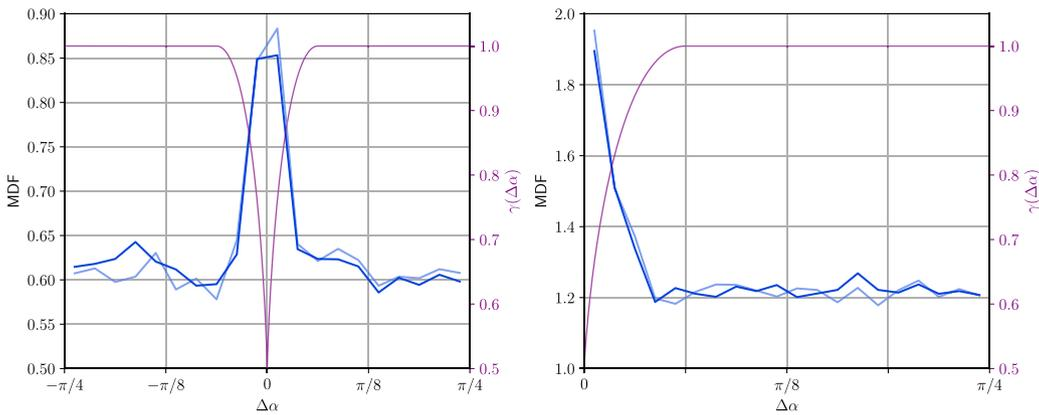
Fig. 19. The Misorientation Distribution Function (MDF) for the Read-Shockley grain boundary energy. The right column accumulates the misorientations for symmetry on  $[0, \pi/4]$ . Light-blue lines correspond to  $\kappa = 1$  and blue lines correspond to  $\kappa = 1000$ .
