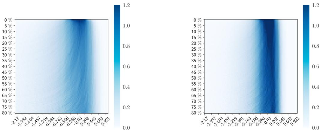
Fig. 13. Evolution over time of relative grain area distribution. The figure on the left corresponds to the numerical experiment performed with  $\kappa = 1$  and the figure on the right corresponds to  $\kappa = 10,000$ . In both cases we used  $\epsilon = 0.2$  for the grain boundary energy. For the cases with  $\epsilon = 0$  and  $\epsilon = 0.02$  the figures look alike so they were not included.
