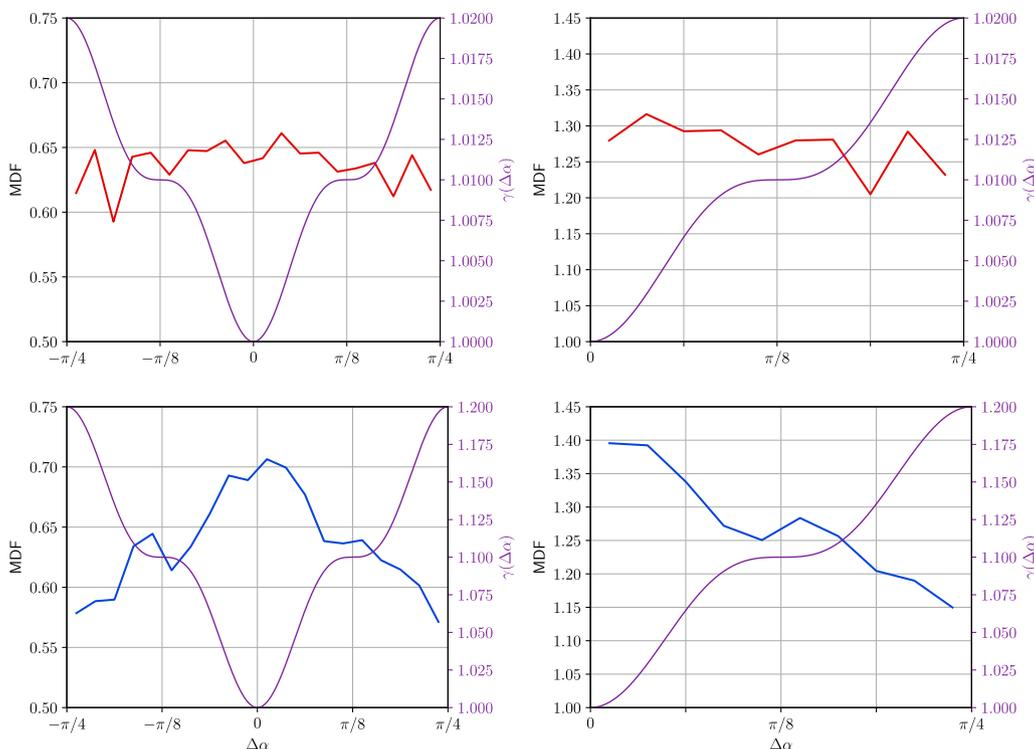
**Fig. 10.** The Misorientation Distribution Function (MDF) for  $\epsilon = 0.02$  (first row) and for  $\epsilon = 0.2$  (second row). The right column accumulates the misorientations for symmetry on  $[0, \pi/4]$ .
