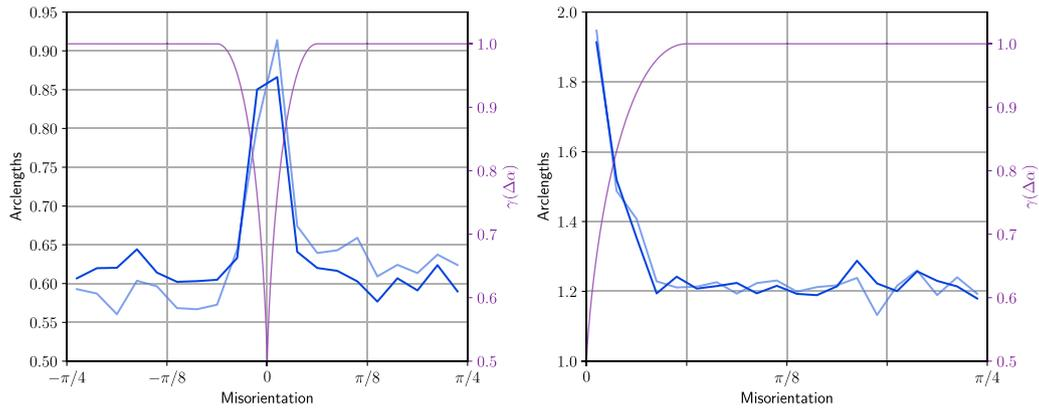
Fig. 18. The Grain Boundary Character Distributions (GBCD) for the Read-Shockley grain boundary energy. The right column accumulates the misorientations for symmetry on  $[0, \pi/4]$ . Light-blue lines correspond to  $\kappa = 1$  and blue lines correspond to  $\kappa = 1000$ .
