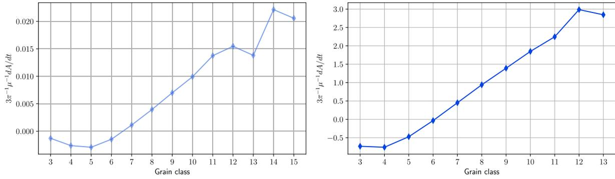
Fig. 17. Rate of change of area per grain class. (Left) Median of  $dA/dt$  for  $\kappa = 1$ . (Right) Median  $dA/dt$  for  $\kappa = 1000$ . This uses the Read-Shockley grain boundary energy.
