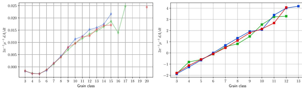
Fig. 7. Rate of change of area per grain class. (Left) Mean of  $dA/dt$  for  $\kappa = 1$ . (Right) Mean  $dA/dt$  for  $\kappa = 10,000$ . This was computed by removing less than 10% of extreme values per class.
