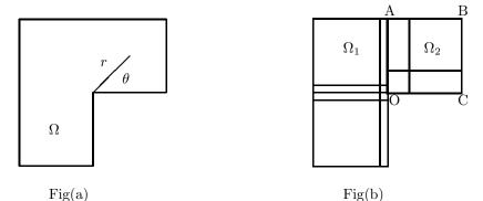
FIGURE 2. (a) L-shaped domain (b) Tensor product mesh for m = n = 2
