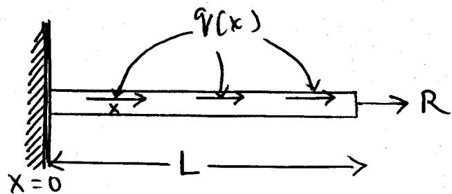
$q(x)$  : DISTRIBUTED AXIAL LOAD (Force per unit length)
