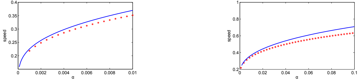
Figure 6: Speed associated to the mean arrival times in numerical simulations on an Erdős Rényi graph with N = 60,000 and expected degree k_{ER} = 2 are shown in asterisks. The blue curve is the spreading speed predicted by the analysis in Section 2 for the homogeneous tree with k = 2.54 , found by numerically computing roots of (2.3). This value is chosen since it is one less than the mean degree of the network over those nodes with distance between 3 and 12 from the original location.
