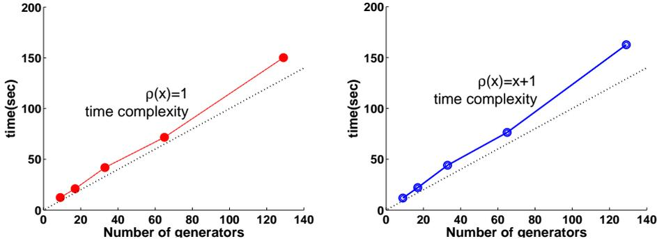
FIG. 4.2. Computational time vs. problem size for the 1d implementation.
