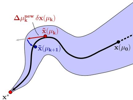
Figure 4. Correction step of the adaptive continuation method.
