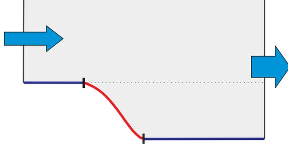
Figure 1. Channel with a backward facing step
