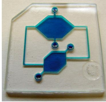
Figure 7. Surface Acoustic Wave (SAW) driven microfluidic biochip
