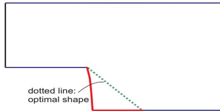
Figure 5. Initial and optimal shape of the backward facing step.
