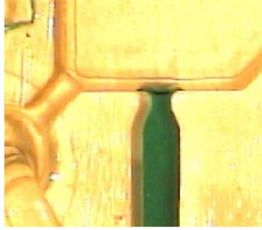
Figure 8. Channel with capillary barrier on an SAW driven microfluidic biochip
