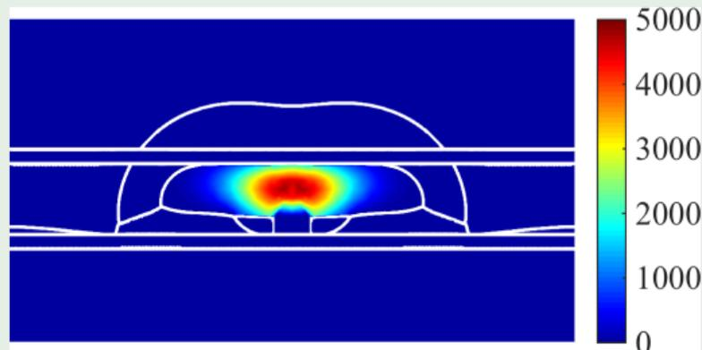
Figure: current-gain characteristics of initial and optimized device (l.) modal gain  $g|\Theta|^2$  [ $\text{cm}^{-1}$ ] optimized design (r.)
