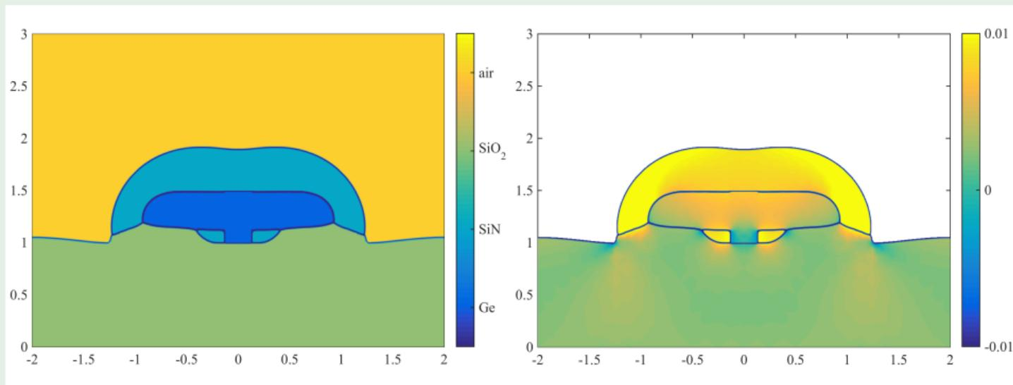
Figure: Optimal material layout (l.) and its corresponding strain field (r.).
