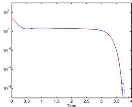
Integrals  $\int_{U_2} u_*^2(x, t) dx$  (solid blue line) and  $\int_{U_2} \hat{u}_*^2(x, t) dx$  (dashed red line) of the optimal controls computed using the full and the reduced order model.
