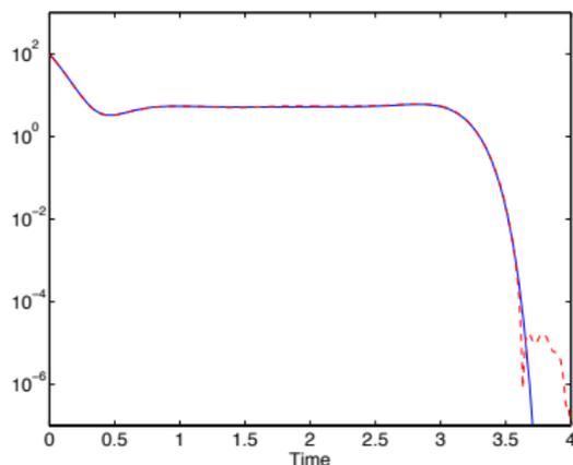
Integrals  $\int_{U_1} u_*^2(x, t) dx$  (solid blue line) and  $\int_{U_1} \hat{u}_*^2(x, t) dx$  (dashed red line) of the optimal controls computed using the full and the reduced order model.
