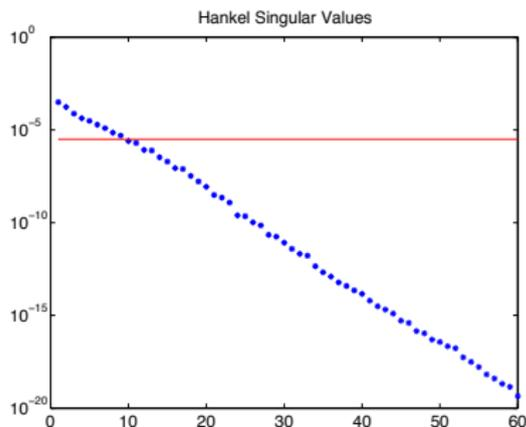
The largest Hankel singular values and the threshold  $10^{-4}\sigma_1$  (fine grid)
