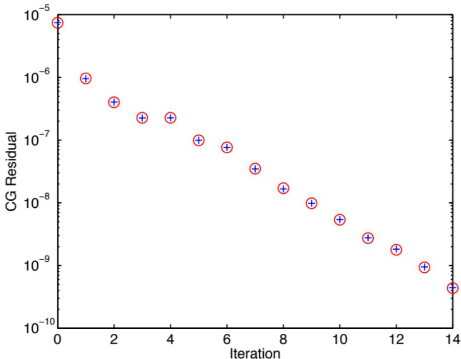
The convergence histories of the Conjugate Gradient algorithm applied to the full (+) and the reduced (o) order optimal control problems.
