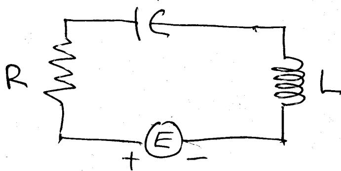
$Q(t)$  = charge on capacitor at time  $t$  initial charge
