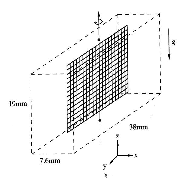
Figure 2: This figure shows the model configuration filled with a stratified fluid. The dimensions are  $0 \le x \le a_x$ ,  $0 \le y \le a_y$  and  $-L \le z \le L$  where  $a_x = 7.6$ mm,  $a_y = 38$ mm and L = 9.5mm are the values corresponding to the experiment by Berg *et al.* The paddle, which in the experiments creates the initial disturbance, is shown for reference and is not present in the mathematical model.
