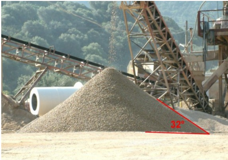
Figure: Gravel pouring from a “point” source (left). Angle of repose of several materials (right)
