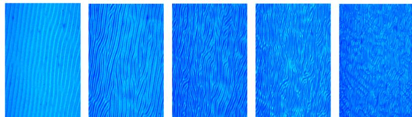
Liquid crystal driven at 10V, 12V, 14V, 16V, and 20V (left to right).
