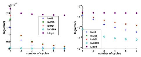
$\rm FIG.~4.5.$  (a) Convergence history for the multigrid scheme compared to the Lloyd scheme shown on the top curve in the normal scale (left) and log-normal scale (right).
