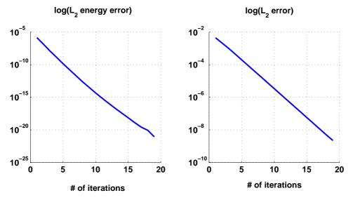
FIG. 4.3. The energy reduction (left) and the convergence history (right) for 129 generators in the log-normal scale.
