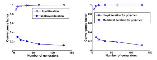
FIG. 4.1. Plot of the convergence factor vs. the number of generators for the regular Lloyd (upper) and the multilevel (lower curves) iterations for  $\rho(x) = 1$  (top) and  $\rho(x) = 1 + 0.1x$  (bottom).
