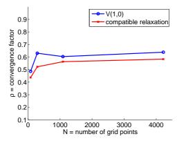
$\rm FIG.~4.4.$  Comparison of the convergence factors for the compatible relaxation and a V(1,0) cycle.
