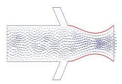
Figure 10. Velocity field for the optimal configuration when the barrier is not in stopping mode
