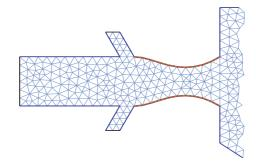
Figure 9. Optimal shape of the capillary barrier and underlying finite element mesh
