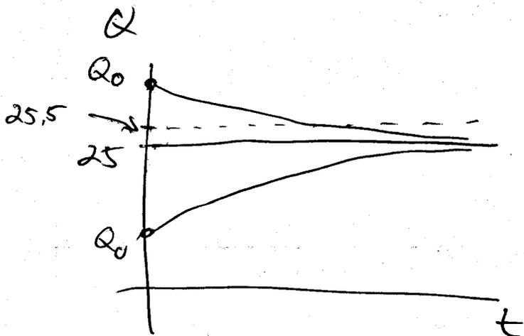
$$(b) Q_0 = 2Q_L = 50 \text{ lb} \quad r = 3 \text{ gal/min}$$
